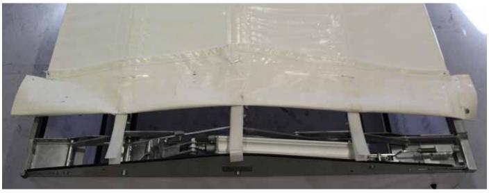
Begin with inserting the plastic strips into the pocket for the tube, the middle plastic strip shall go outside the gable, as seen on the picture.
