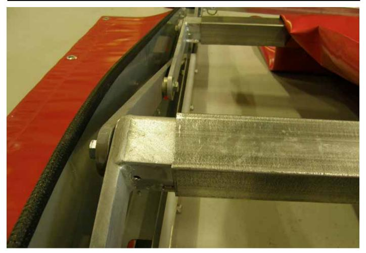
When the outer tubes are mounted, the inner tubes can be in need of some adjusment. when the outer tubes is fixed, the outer tubes shall be drilled and screwed, first check that all the arms are parallel, if not this should be corrected.
