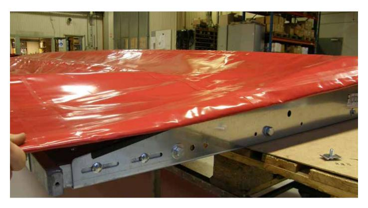
Center the tarpoulin, equal overhang front and rear, and an equal measure of the sides.
