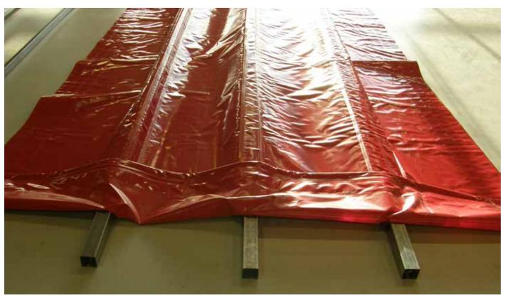
Place the tarpoulin with the outside up and push in the three 60x60x2 tubes with tape ends first. (not to damage the fabric)
