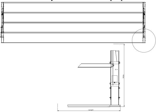
Adjust the width of the end pieces by first adjusting the fixed side. Then cut the tubes (60x60x2 4pc and 50x30x2 1pc) Length = L - 330mm at one cylinder. When two cylinders is the deduction Length = L - 440mm.
