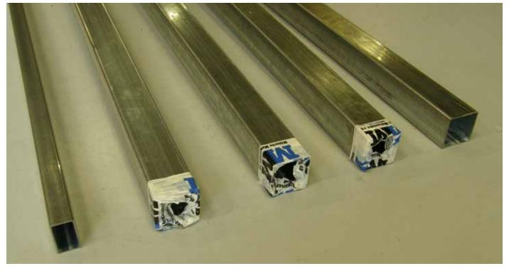
Remove burrs from the pipes inside and outside, and tape 3 of 60x60x2 tubes like the picture above
