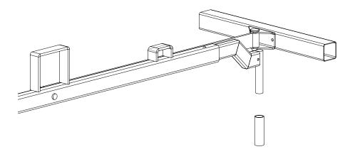
Therafter adjust the arc support so that the side tube is in line with the platforms outer surface and tarpoulin tensioned. Drill and screw down the bow on both sides.
