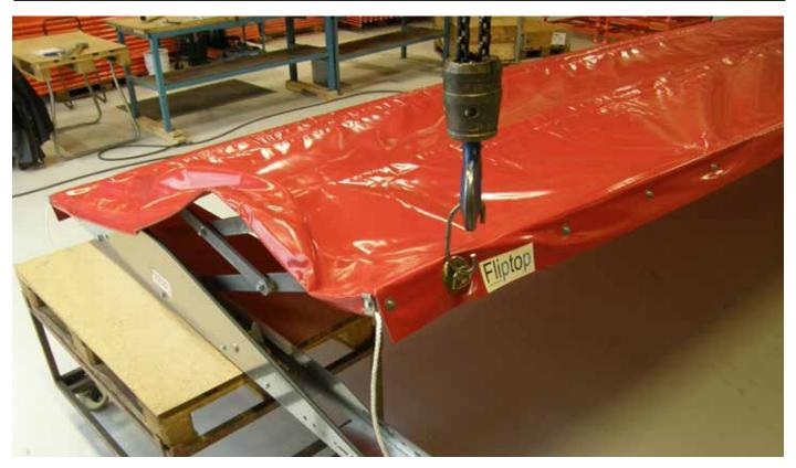
The easiest way to stretch the rope is to open the gable about  $100~\mathrm{cm}$ , fasten the rope with the rope clamps. Then cut the rope to fitting lenght
