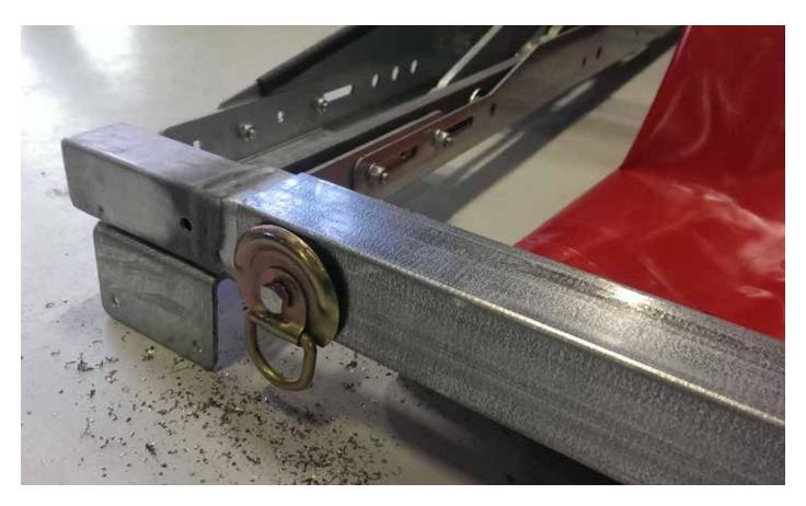
The side with 60x60x2 shall be mounted with M10x75 (1pc), Tie down clamps (1pc) and M10 locknut (1pc).
