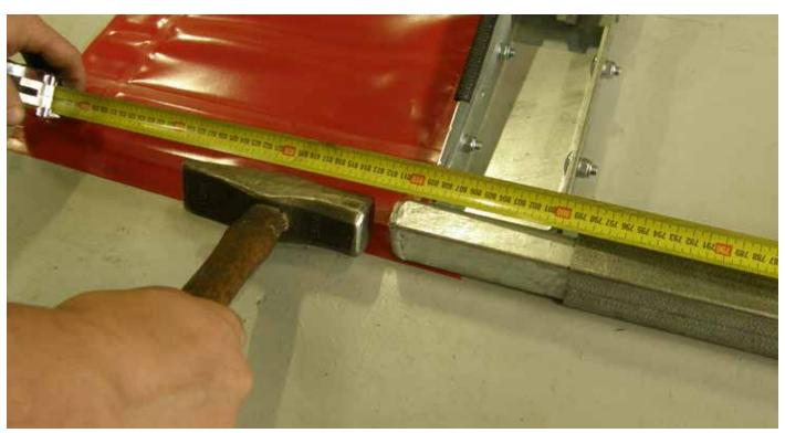
Be very careful when measure the distance before drilling holes and mounting it togheter. The side with 50x30x2 steel tube shall be mounted with M10x45 (1pc) and a M10 locknut (1pc). NOTE! Dont screw the bolts to tight, cause they will be taken out and back again when the tarpoulin will be mounted.
